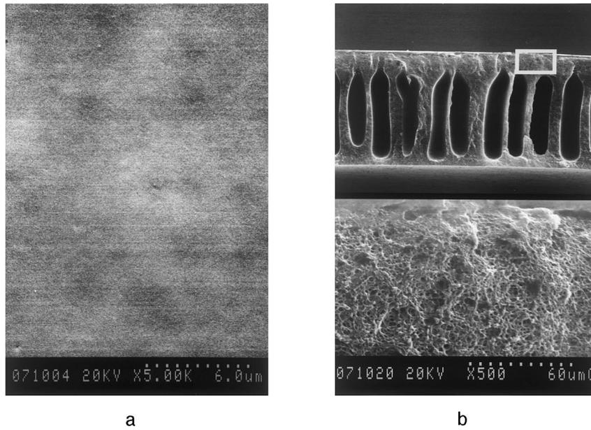
Fig. 4. SEM photomicrographs of membrane from a 15 wt.% of EVAL solution immersed in water without the evaporation step. (a) Top surface; (b) cross-section.
