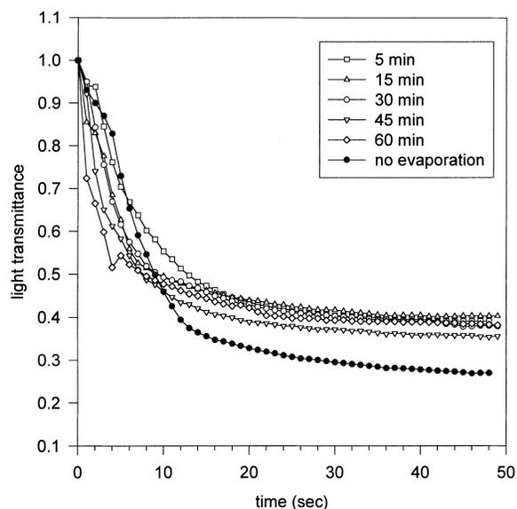
Fig. 3. Light transmittance profiles for precipitation of a 15 wt.% EVAL solution in a water bath after various solvent evaporation times.
