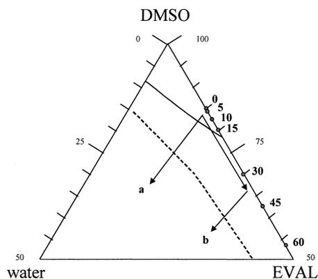
Fig. 8. Composition paths for precipitation of a 15 wt. % EVAL solution in a water bath (—: crystallization equilibrium line; ---: binodal boundary). (a) without evaporation; (b) with evaporation. The numbers shown denote evaporation time.
