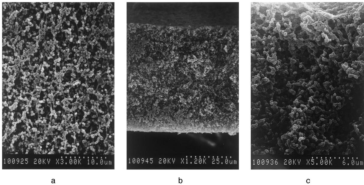
Fig. 7. SEM photomicrographs of membrane from a 15 wt.% of EVAL solution immersed in water after 60 min of evaporation. (a) Top surface; (b) cross-section; (c) magnification of (b).
