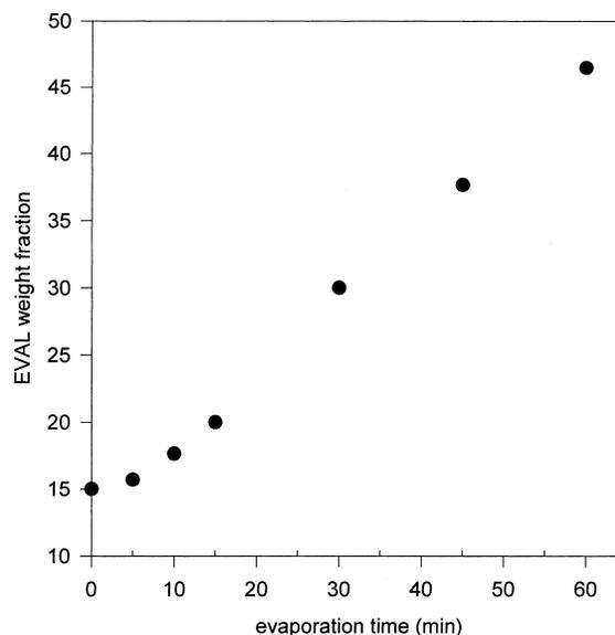
Fig. 2. EVAL weight fraction of a 15 wt.% EVAL solution after various solvent evaporation times.
