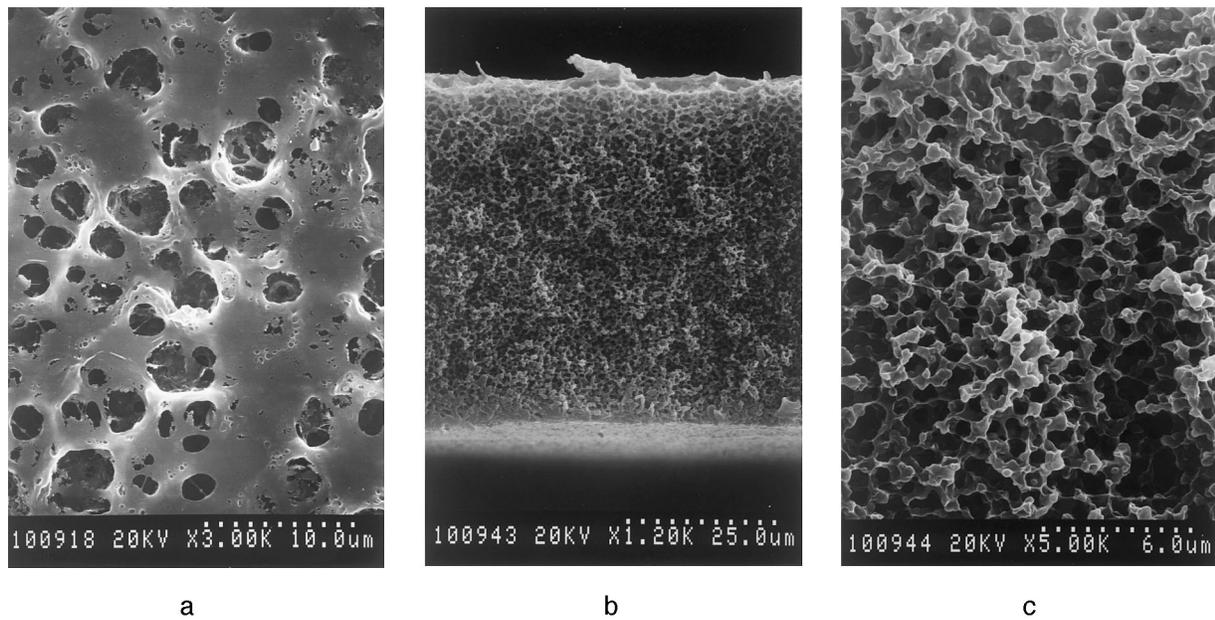
Fig. 5. SEM photomicrographs of membrane from a 15 wt.% of EVAL solution immersed in water after 30 min of evaporation. (a) Top surface; (b) cross-section; (c) magnification of (b).
