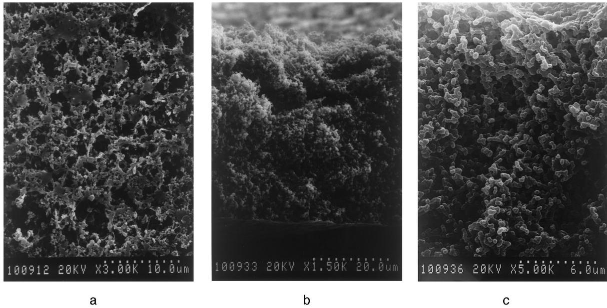
Fig. 6. SEM photomicrographs of membrane from a 15 wt.% of EVAL solution immersed in water after 45 min of evaporation. (a) Top surface; (b) cross-section; (c) magnification of (b).
