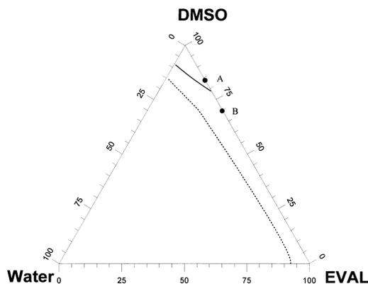
Fig. 1. Phase diagram of water-DMSO-EVAL at 25°C [8]. (—: crystallization equilibrium line;---: binodal boundary).
