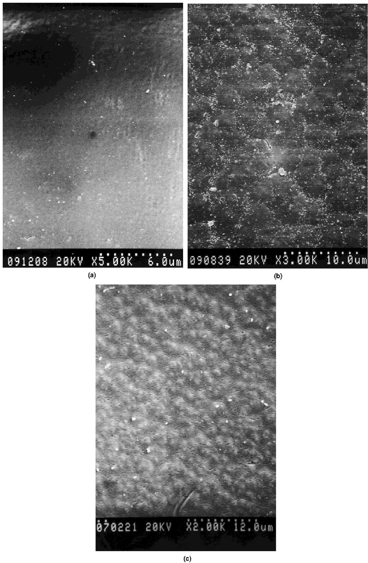
**Figure 1.** SEM photographs of nonporous surfaces of (a) PEVA, (b) Nylon-66, and (c) PVDF.
