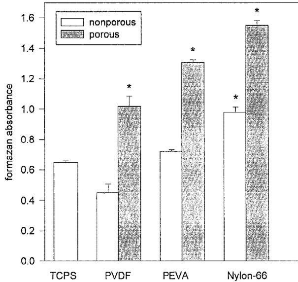
**Figure 3.** The formazan accumulation at 24 h from monocytes seeded onto membranes and TCPS ( $n = 4$ ). \*Significant differences ( $p < 0.05$ ) of monocyte adhesion compared to TCPS.
