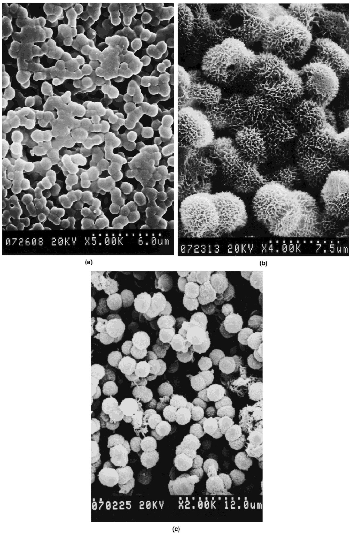
Figure 2. SEM photographs of porous surfaces of (a) PEVA, (b) Nylon-66, and (c) PVDF.
