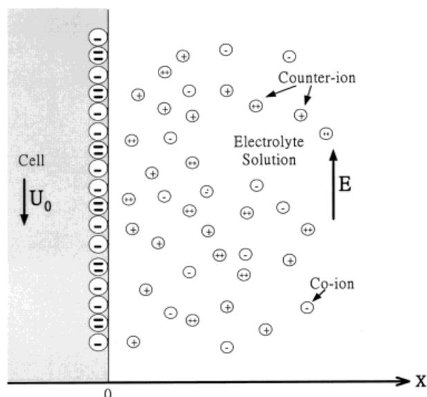
**Figure 1.** Schematic representation of the problem considered. An electric field  $E$  parallel to the surface of a cell is applied,  $U_0$  is the electrophoretic velocity of the cell, and  $X$  is the scaled distance from cell surface.
