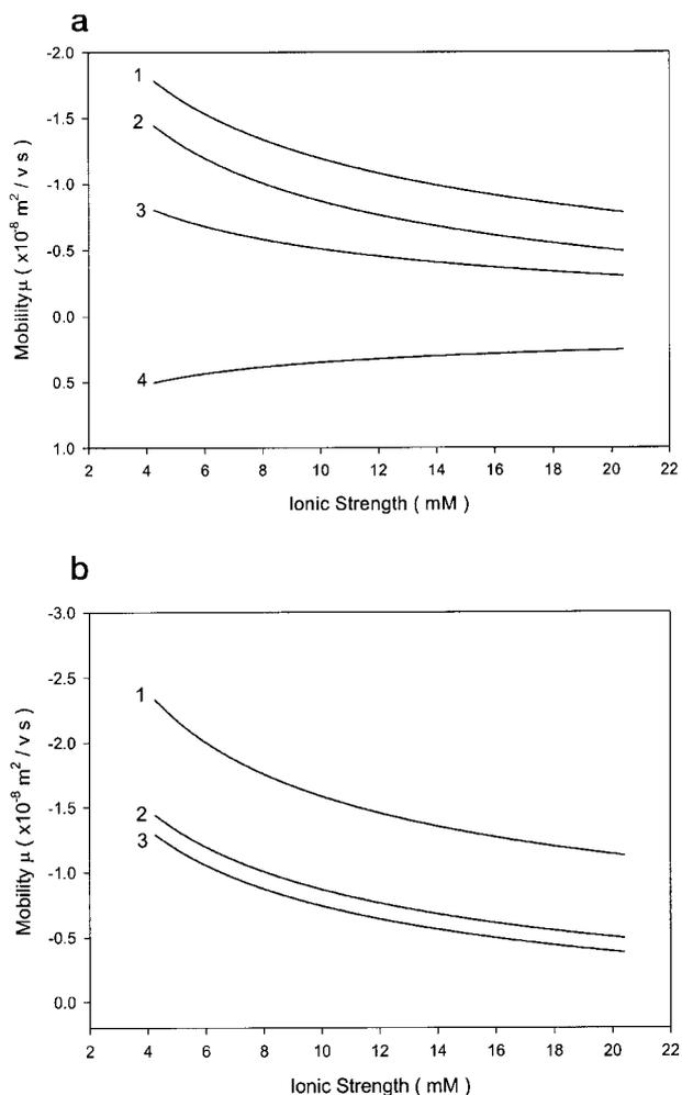
**Figure 5.** Variation of cell mobility  $\mu$  as a function of ionic strength for the case of  $N_{sa} = 5.0 \times 10^{-8}$  mol/m<sup>2</sup>,  $N_{sb} = 5.0 \times 10^{-8}$  mol/m<sup>2</sup>,  $K_{a1} = 1.0 \times 10^{-5}$  M,  $K_{a2} = 1.0 \times 10^{-9}$  M,  $K_{m1} = 50$  M<sup>-1</sup>,  $K_{m2} = 0$  M<sup>-1</sup>,  $K_b = 3.0 \times 10^{-12}$  M. (a)  $\xi = 0.615$ , curve 1, pH 9; 2, pH 7; 3, pH 5; 4, pH 3. (b) pH 7, curve 1,  $\xi = 0$ ; 2,  $\xi = 0.615$ ; 3,  $\xi = 1$ .
