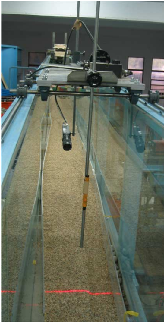
Figure 2. Photograph showing the experimental setup and DTM scanning system. Shown in the front is the laser sheet projected on the bed and the resulting distorted laser line.
