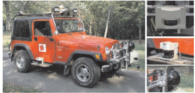
Fig. 2. Right: the Navlab11 testbed. Left: SICK LMS221, SICK LMS291 and the tri-camera system.
