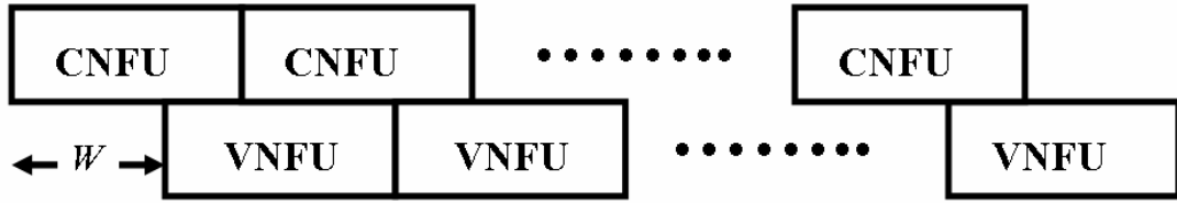
Fig. 3. Overlapped Pipelining of check node's and variable node's function units
