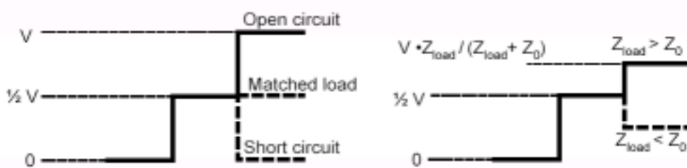
Fig. 4 Typical TDR waveform( V_{measured} ).
