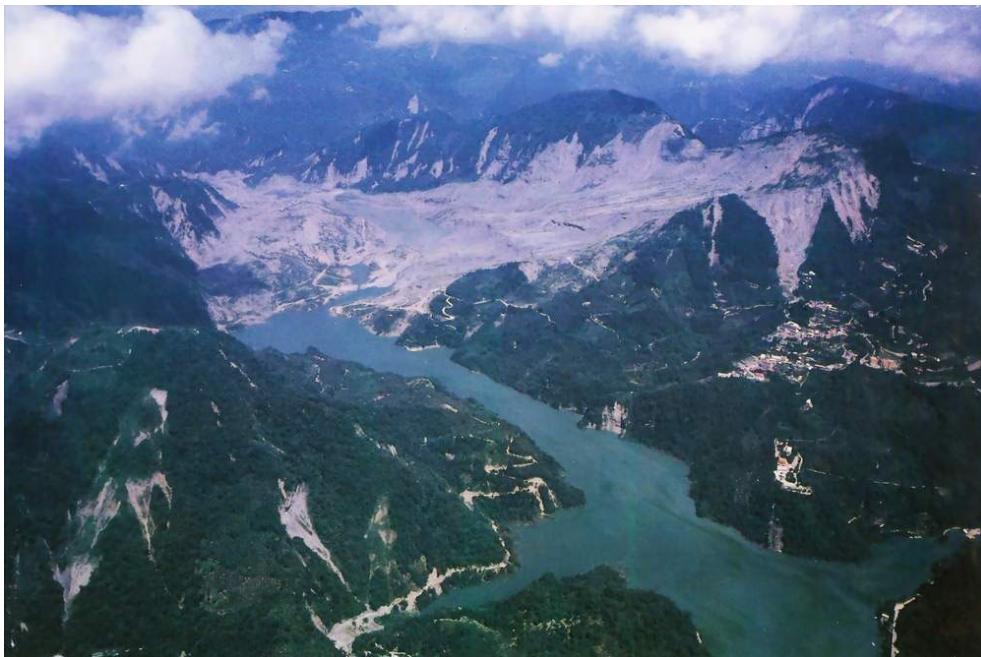
Figure 19. Aerial view of the Tsaolin Landslide Dam and Lake seen from upstream, shortly after the 1999 Chi-chi Earthquake. (Source: Lai C.H.)
