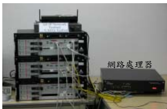
圖二十三：All-IPv6 Network Testbed and Network Processor
