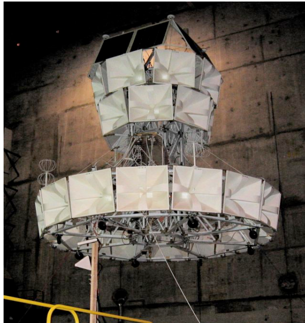
Fig. 3 The ANITA detector in SLAC's End Station A (ESA) ready for calibration of the Askaryan Cherenkov radiation from ice (June 2006).
