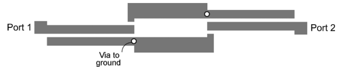
Fig. 9. Layout of the fourth-order microstrip coupled-line bandpass filter in [16].
