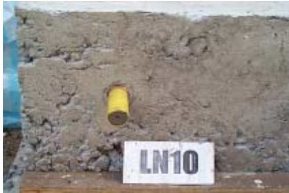
Figure 6 Appearance of NC-C-10 (normal concrete, vibration against rebar for 10 seconds)
