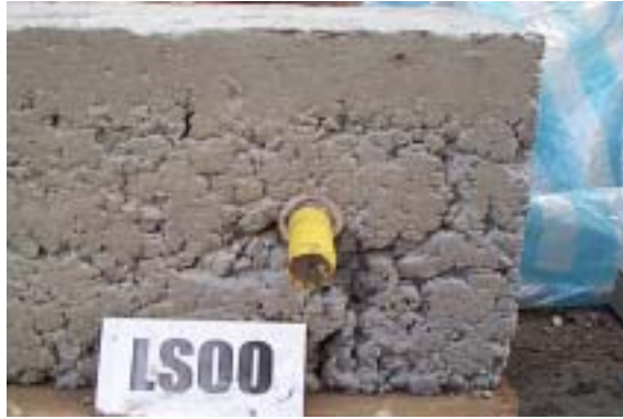
Figure 5 Appearance of Specimen NC- 00 (normal concrete, no vibration)
