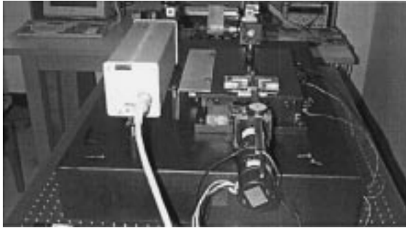
Fig. 16. Precision ball-screw table with laser scale.
