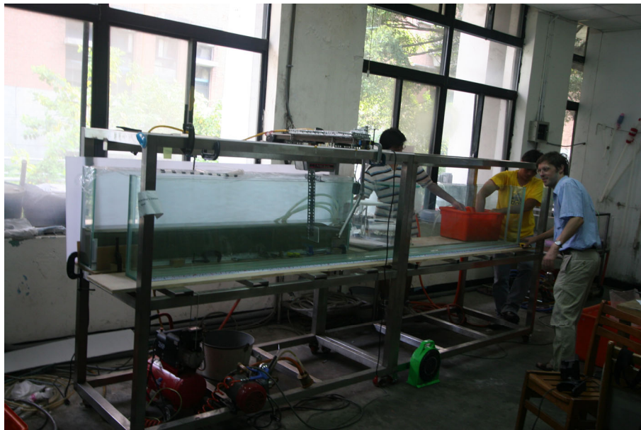
Figure 3. Laboratory tank used for the study of underwater jet trenching flows.
