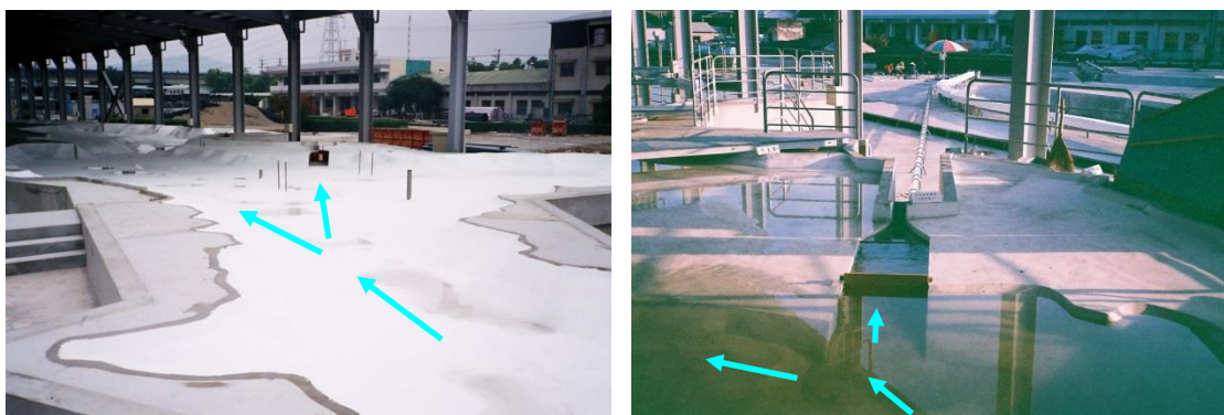
Fig. 7: The model of Project D2 model and simulation test of Typhoon Aere in Project D2
