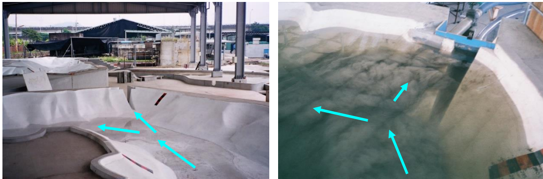
Fig. 6: The model of Project C with extending pipe model and simulation test of Typhoon Aere in Project C with extending pipe
