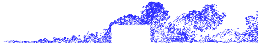
Figure 9: Numerical simulation of a uniform flow passing a rectangular dike (time = 30.0 sec)
