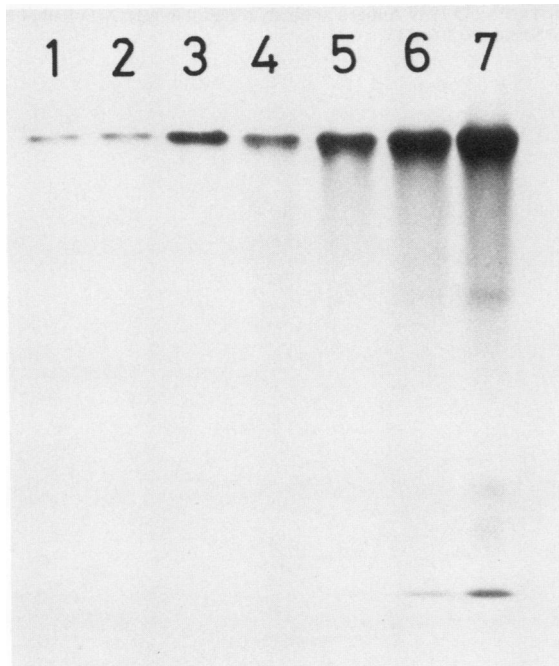
FIG. 2. Disc PAGE patterns of purified SPI and a commercial BA in 7.5% gel (pH 8.3). Lanes 1 to 3 contained 1.5, 2.5, and 5 \mu g of purified SPI; lanes 4 to 7 contained 3, 5, 15, and 30 \mu g of Sigma BA, respectively, and were stained with Coomassie blue R.
