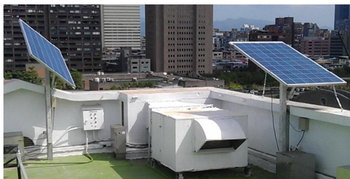
Fig. 1. Comparative test of 1A-3P sun tracking PV.
