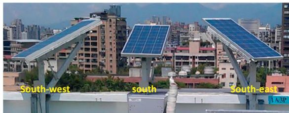
Fig. 3. Comparative test on the effect of misalignment of 1A-3P installation direction.
