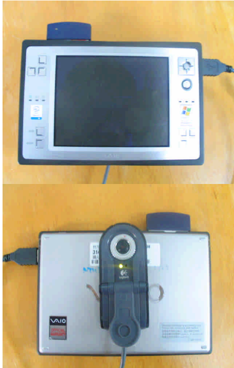
Fig 5 The Camera consist of a Palmtop PC and a Logitech Webcam
