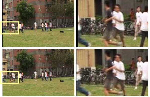
Fig. 6: Upper-Left: The frame after changing the position according to the stabilized camcorder motion path. There is a missing area at the left side and a moving object across the missing area. Lower-Left: The result of dynamic region completion. Right Column: The close up view of the yellow square of the Left Column.
