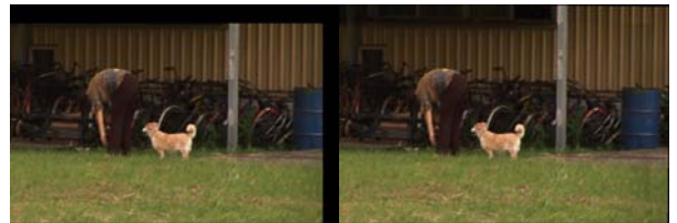
Fig. 8: Left: The frame after changing the position according to the stabilized camcorder motion path. There is a missing area at the right side and upper side. Right: The result of static region completion. Since the missing area is large, there is a discontinuity boundary between the recovered pixels and the original frame.
