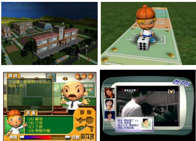
Figure 5: Some snapshots of MPEG-4 applications. The first three pictures is a MPEG-4 game. This game mixed 2D and 3D within a single scene, and using JavaScript to control the logical interaction. The last picture is a MTV scene and contains some videos.
