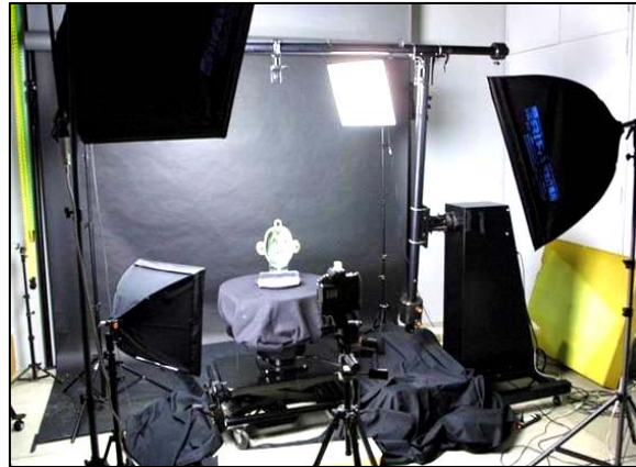
Fig. 4: Acquisition of Object Movies with autoQTVR.
