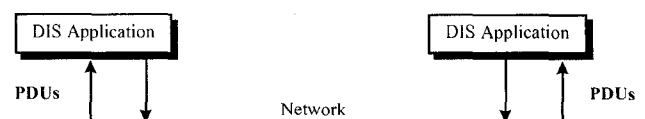
Figure 4 The control flow of DIS. A DIS application needs to maintain all the simulation information necessary, and uses PDUs to communicate with each other.
